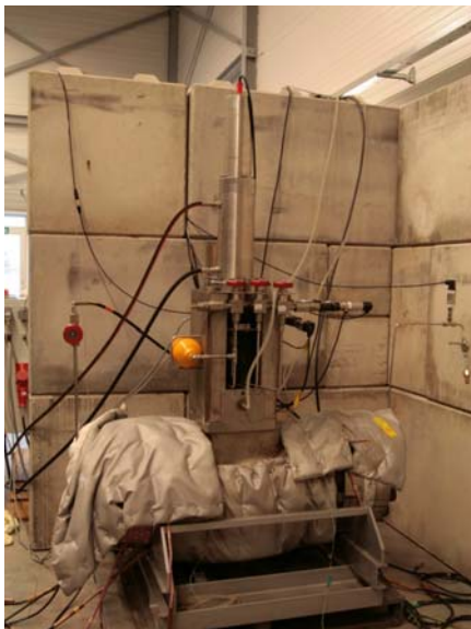
valve endurance testing
