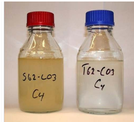
Figure 6: Separator water outlet OiW concentration as a function of WC and valve type (left), water samples from the same test conditions for the standard and Typhoon Valve System (right).
